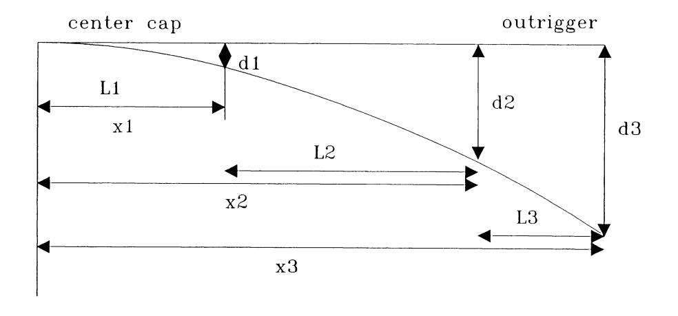
Fig. 1 Profile for 16 um tape x1=150;x2=350;x4=450 vertical scale expanded by factor of 10
