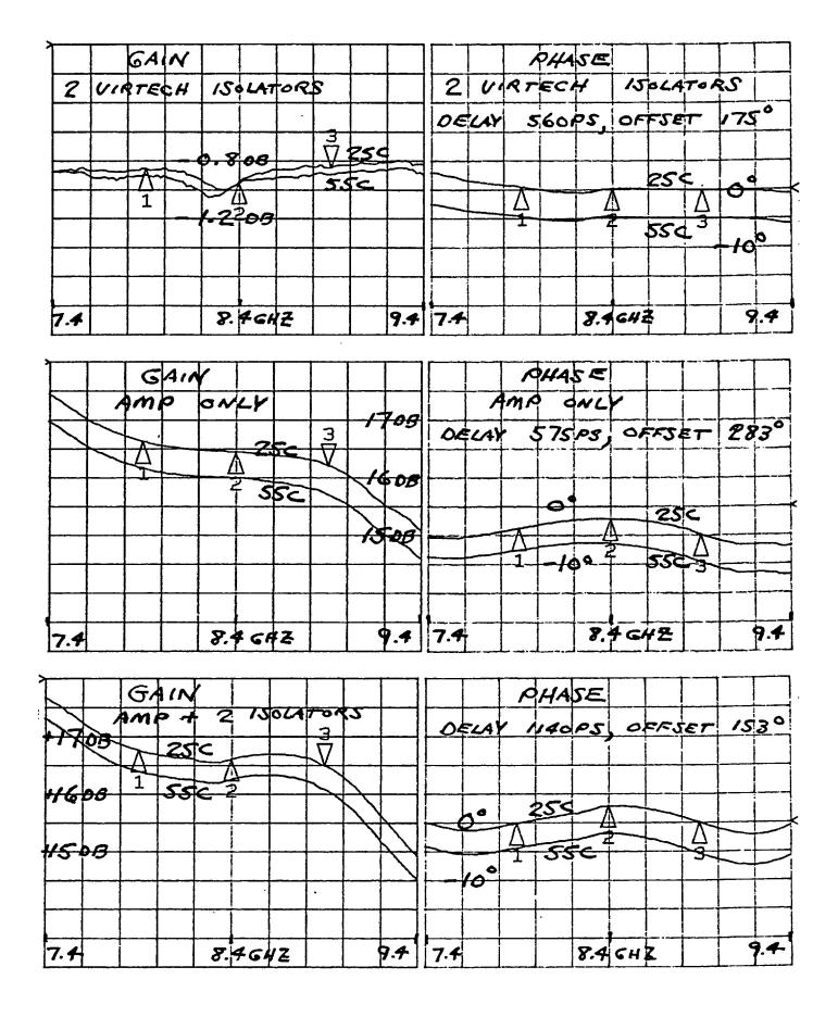
Fig. 3. Test results for X-band isolators and amplifier.
