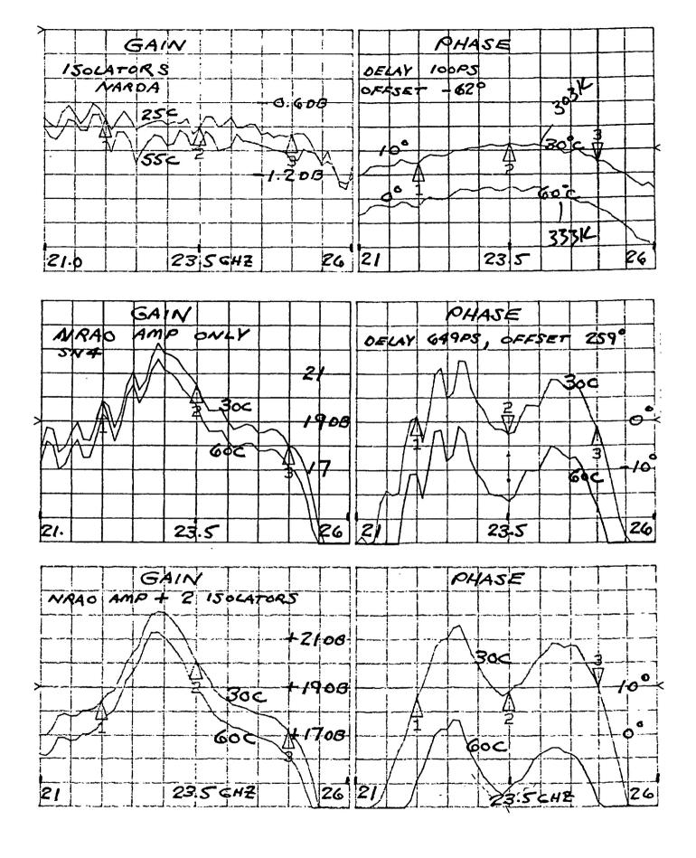
Fig. 5. Test results for K-band isolators and amplifier.
