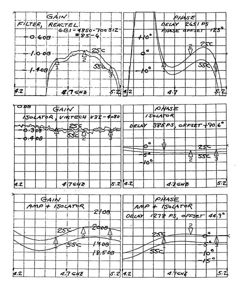
Fig. 2. Test results for C-band filter, isolator, and amplifier.
