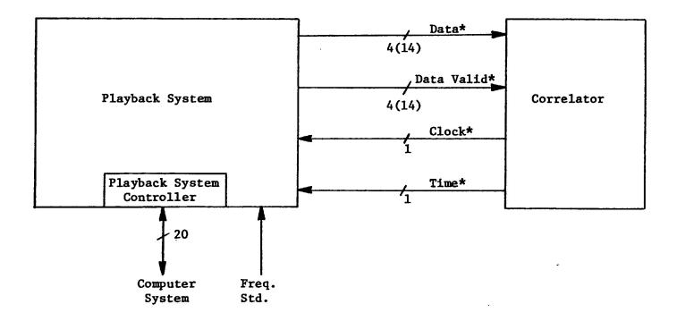
\* ECL differential signal (synchronous with clock).
