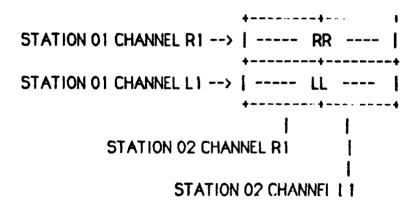
NP processing requires no combination of the R and L channels, so double the delay coverage and frequency resolution (per channel) are available compared with P mode. Since R and L channels will generally be from separate IF frequencies, two independent lobe rotators are required.
