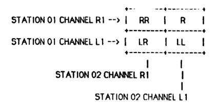
Only one lobe rotator is required for such a group of 4 correlators operating in P mode, since interferometer geometry and frequency are identical for all. Channel-specific (or R/L-specific) delay, phase or frequency offsets can be removed in later processing.
