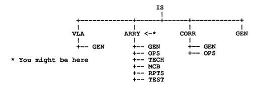
The "IS" section is the top-most level. This section is accessed by starting IS on ZIA or entering the "is" file command when on VLBACC. When IS is started on VLBACC you will normally start out in the ARRY section. The ARRY section contains VLBA-only information. The VLA section is for the VLA, and the CORR section will be for the VLBA correlator. GEN contains general information (mostly for the VLA).
