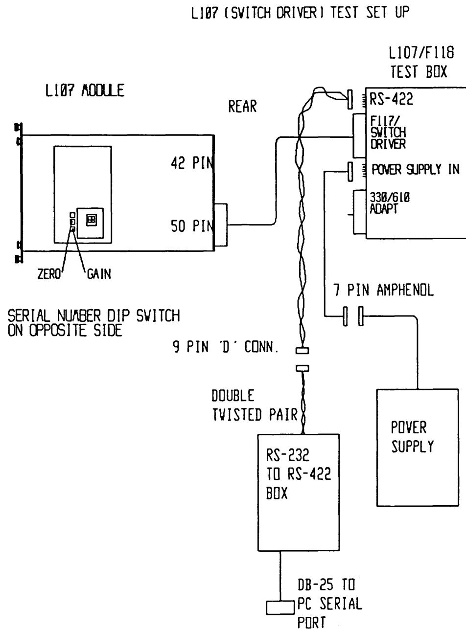
Figure 1. L107 Test Set-up.
