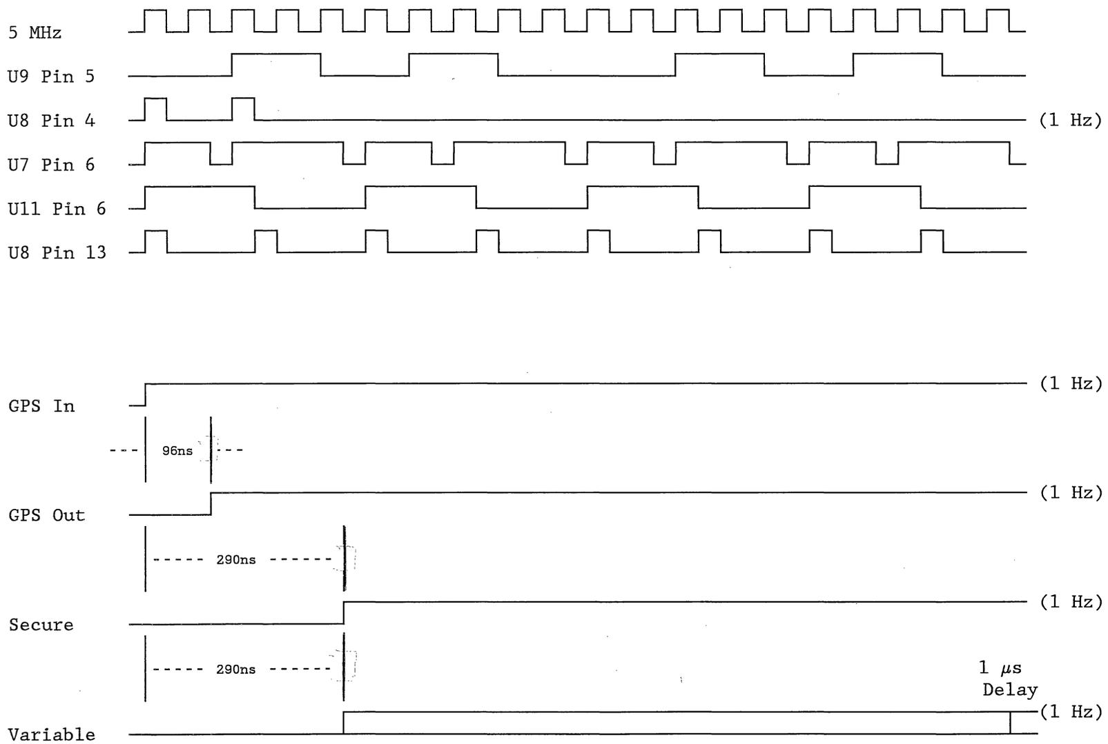
Figure 1: Waveforms of the L109
