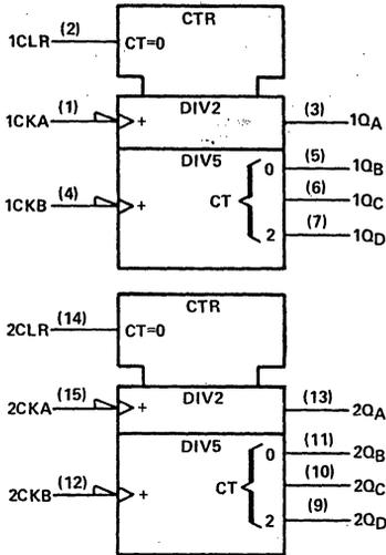
logic diagram, each counter (positive logic)
