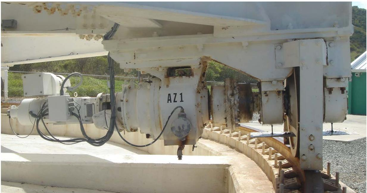
Figure 2, Mark II design wheel/axle assembly.
