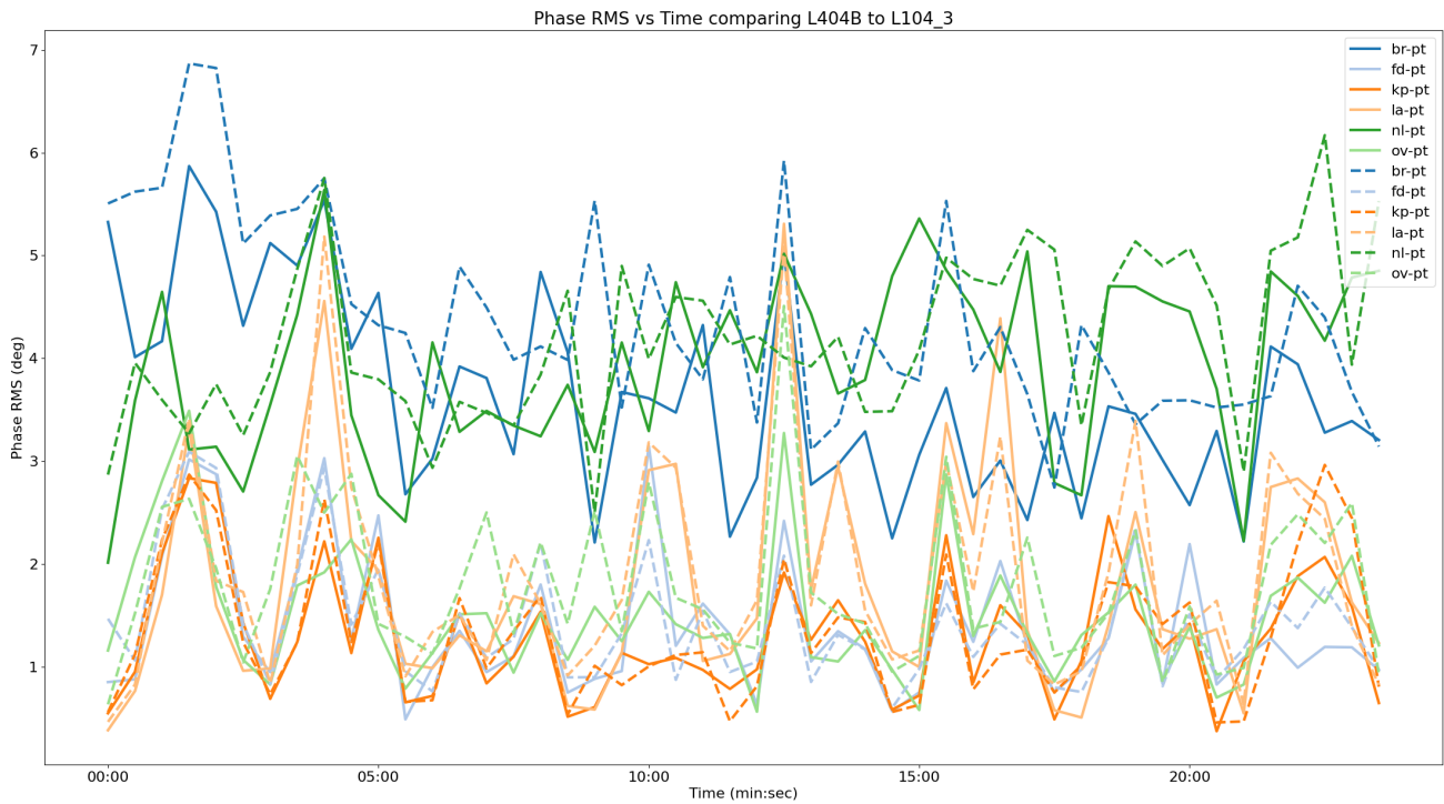
Figure 7: Phase RMS vs time, calculated over 30 second solution intervals, comparing the phase rms of the L404A at Pie Town (solid lines) with the L104.3 (dashed lines) by plotting spectral channel 30 of IFs 1 and 3 respectively. Note the setup ends up with sky frequencies of around 8.2 and 8.8 GHz for the L404A and L104.3 respectively so the data are not quite one to one. Note also these data come from 8, 3 minute scans with gaps removed here.
