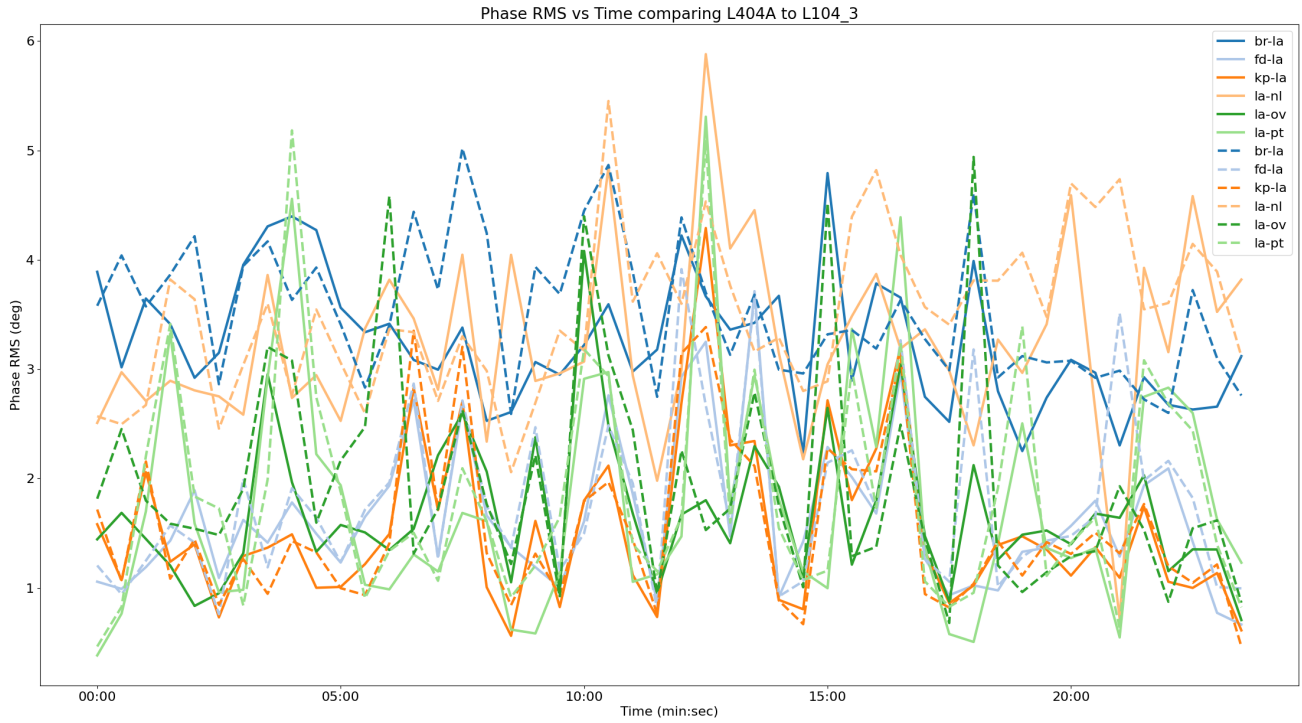
Figure 6: Phase RMS vs time, calculated over 30 second solution intervals, comparing the phase rms of the L404A at Los Alamos (solid lines) with the L104.3 (dashed lines) by plotting spectral channel 30 of IFs 1 and 3 respectively. Note the setup ends up with sky frequencies of around 8.2 and 8.8 GHz for the L404A and L104.3 respectively so the data are not quite one to one. Note also these data come from 8, 3 minute scans with gaps removed here.
