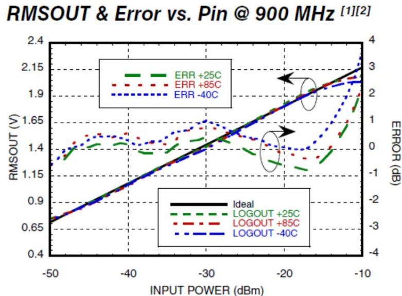
**Figure 3: HMC909LP4 voltage-power response and error function for CW and noise-like signals at 900MHz. Source: Hittite Microwave**
