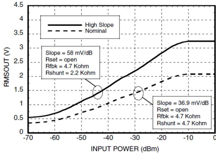
**Figure 4: HMC909LP4 slope adjustment for power magnification.**
