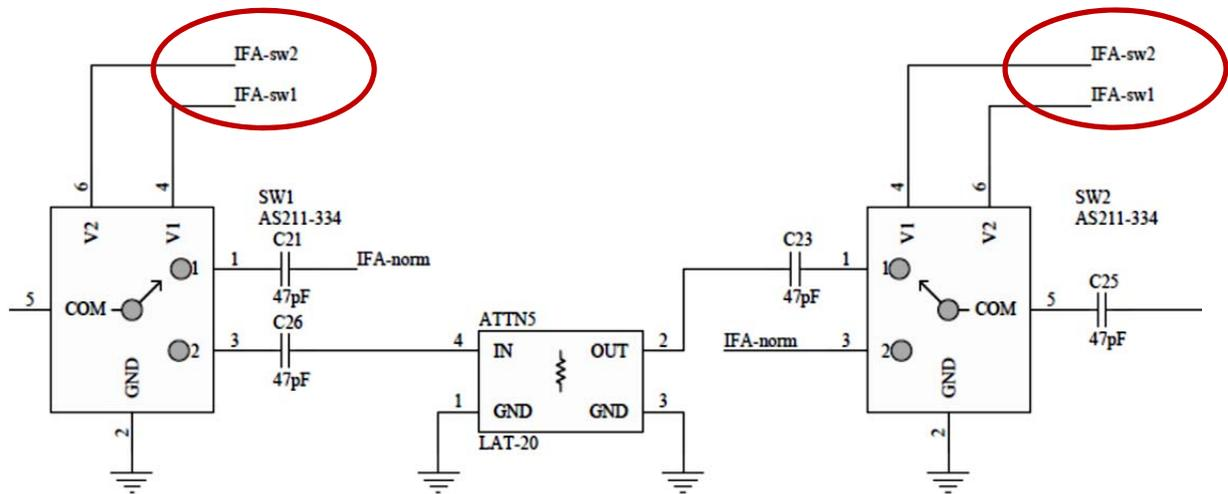
**Figure 6: Schematic detail of IFA circuit, showing redundant complementary solar attenuator control line which can be reconfigured as ADC chip select signals. IFB similarly has a redundant control line.**
