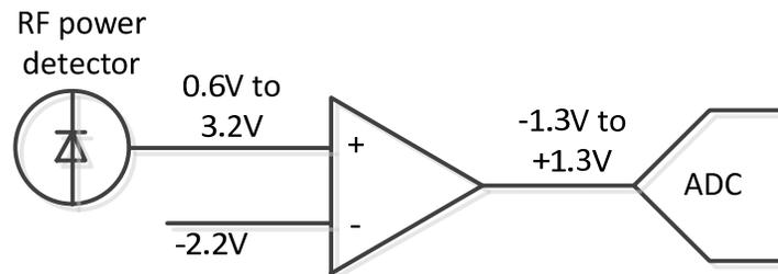
**Figure 5: Voltage-offsetting circuit for detector/ADC interface**
