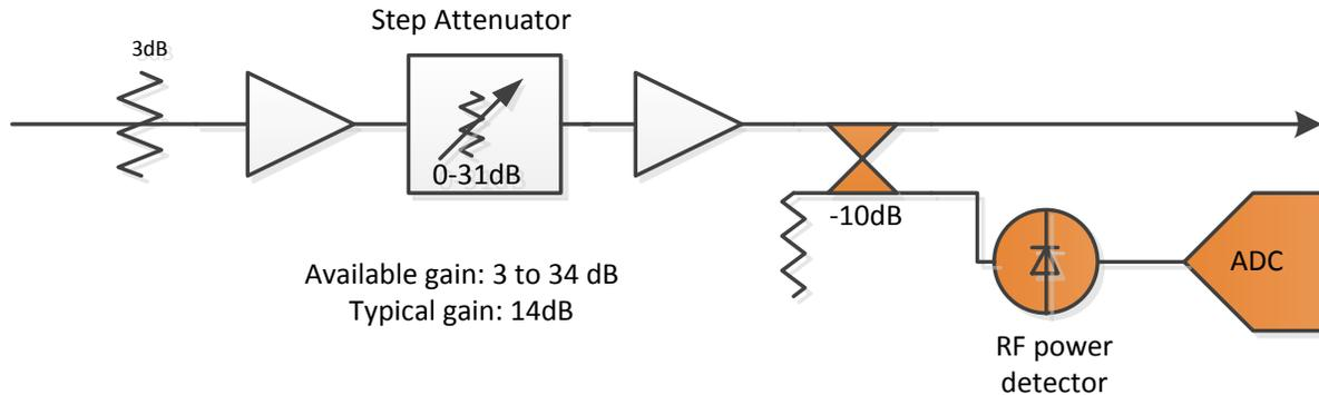
**Figure 1: Functional block diagram of ALC module. The orange-shaded components – coupler, detector, and ADC -- are the new additions to the circuit**
