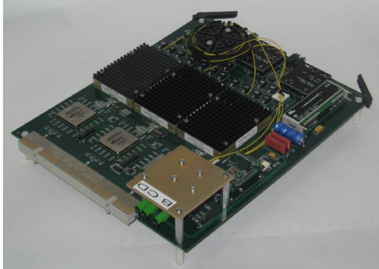
Figure C.7. The DRXA. A total of 264 will be installed in the Bilateral Correlator.
