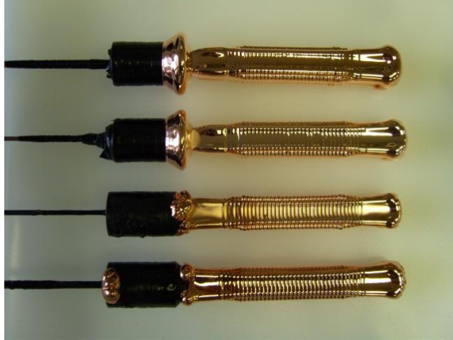
Figure F.16. EVLA K-band phase shifters electroformed using the new process.
