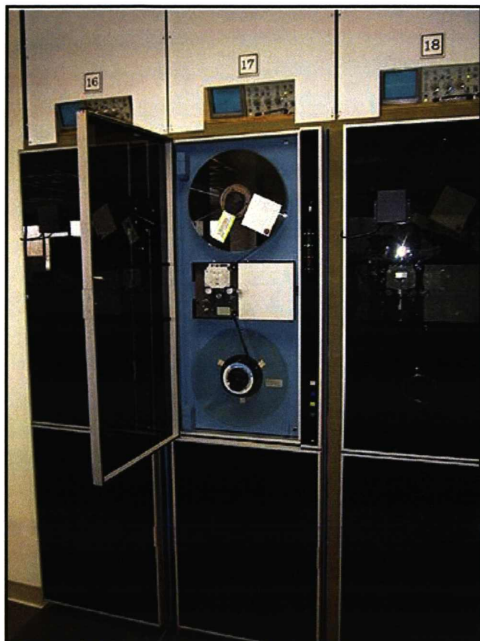
Figure IV.6 A VLBA tape drive, showing one of the many magnetic recording tapes currently in use at the VLBA. One tape holds approximately 590 Gb of data, corresponding to just over 10 hours of recording at 128 Mbits/sec. The original cost of each tape, together with its glass reel, was about $1,300, while the headstack assembly costs roughly $12,000.
