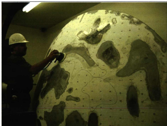
Figure IV.8 An antenna mechanic manually re-surfaces the spare VLBA subreflector to improve its high-frequency performance.
