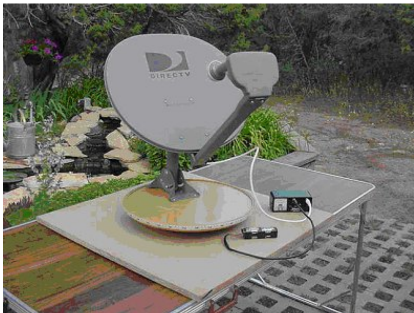
Figure 6. Itty Bitty Radio Telescope constructed by teacher in the Radio Astronomy for Teachers course. (See http://www.aoc.nrao.edu/epo/teachers/ittybitty/procedure.html )
