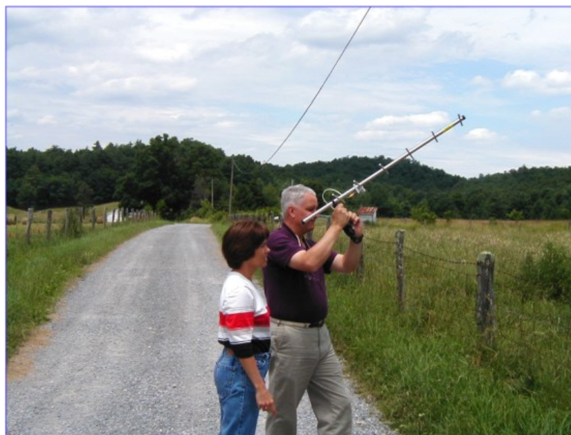
Figure 5. RET teacher Charles Gear checks for power line noise.
