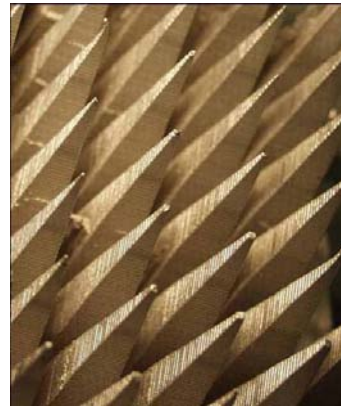
Detail pyramid tips prototype Al casting
