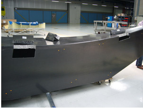
Prototype CFRP BUS Segment showing invasive quality inspection cut-outs
