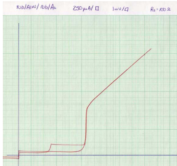
Figure 1. I(V) characteristic of a Nb/Al-AlN/Nb SIS junction with J_C = 30,000 \text{ A/cm}^2
