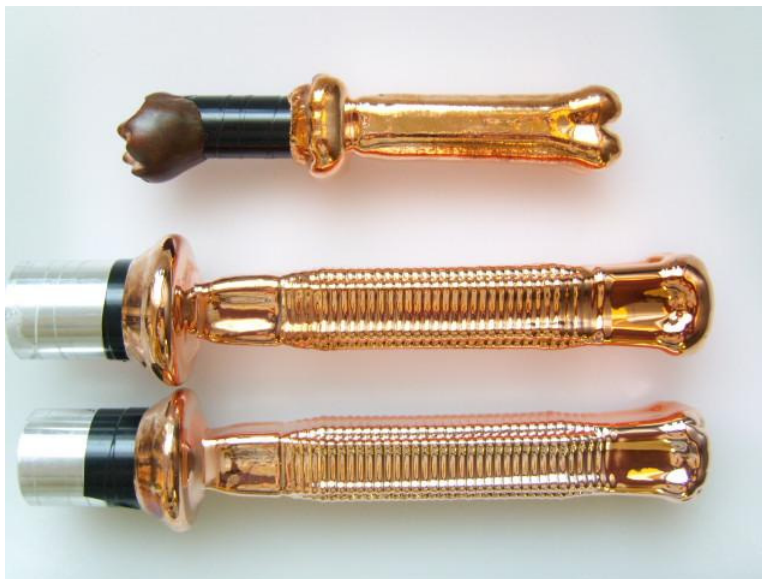
Figure 3. Recently plated copper electroformed phase shifters.
